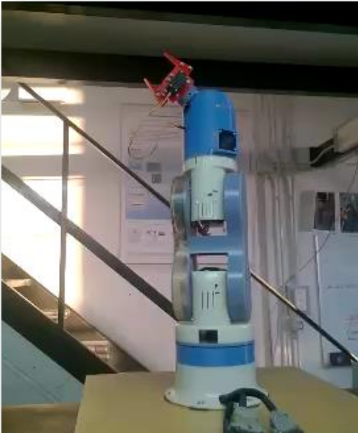
A robotic arm for manipulating different tools for landmine removal
