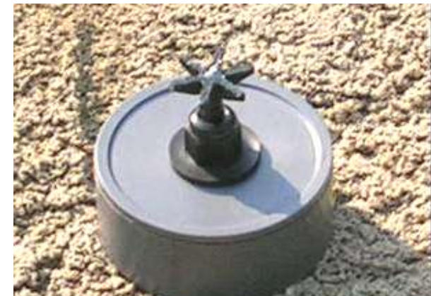
Plastic Mine PMA-2 plastic, Yugoslavia (diameter 68mm, height 61mm, weight 135g)
