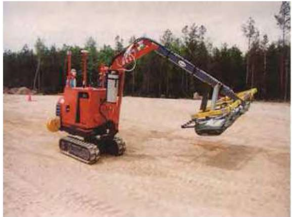
Vehicle Mine Detector (VMMD) with GPR and Metal detectors mounted on the robotic arm.
