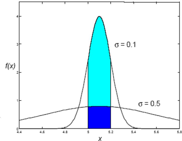
$$\begin{aligned}\mu &= 5.1 & \sigma &= 0.5 \\ X = 5.0 &\Rightarrow Z = \frac{5.0 - 5.1}{0.5} = -0.2 \\ X = 5.2 &\Rightarrow Z = \frac{5.2 - 5.1}{0.5} = 0.2 \\ P(5.0 \leq X \leq 5.2) &= P(-0.2 \leq Z \leq 0.2) = 2[P(Z \leq 0.2) - 0.5] = \\ &= 2(0.5793 - 0.5) = 0.1586 \cong 16\%\end{aligned}$$
