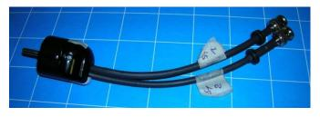
The circuit model of the coupling network and adapter is validated through vector network measurements.
