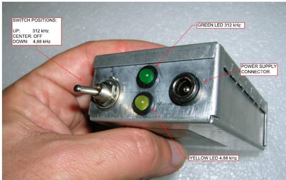
Fig. 3: Detail of the comb generator.
