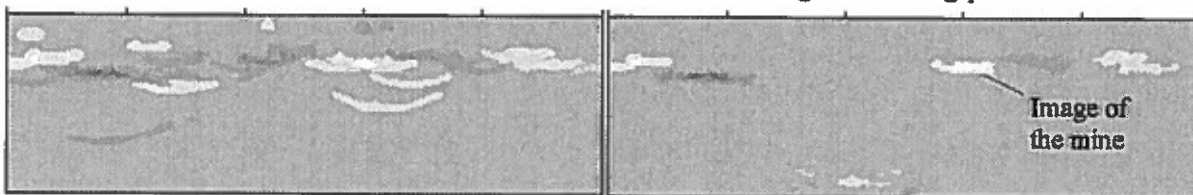
a) Result of 2-dimensional focusing b) Focusing with the selecting and testing of objects Fig.4 Results of focusing for neighboring line of motion of antennas.
