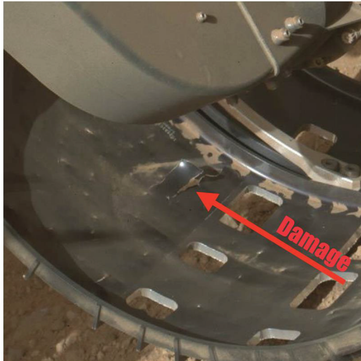
Figure 2. Detail view of the inner surface of Curiosity's left front wheel on sol 411. Arrow points to tear.
