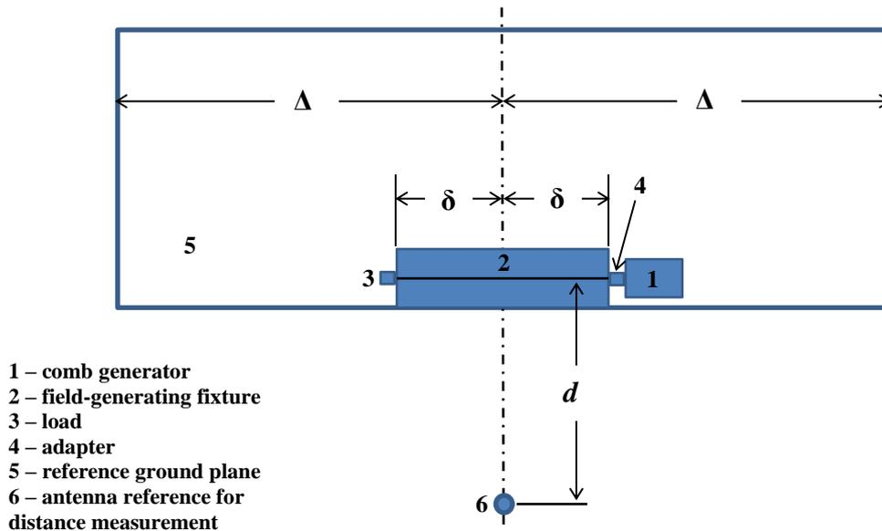
**Fig. 4:** Measurement setup.
