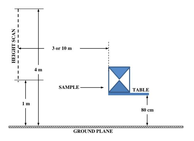
30 to 1000 MHz frequency rage, semi-anechoic room (3 or 10 m)
