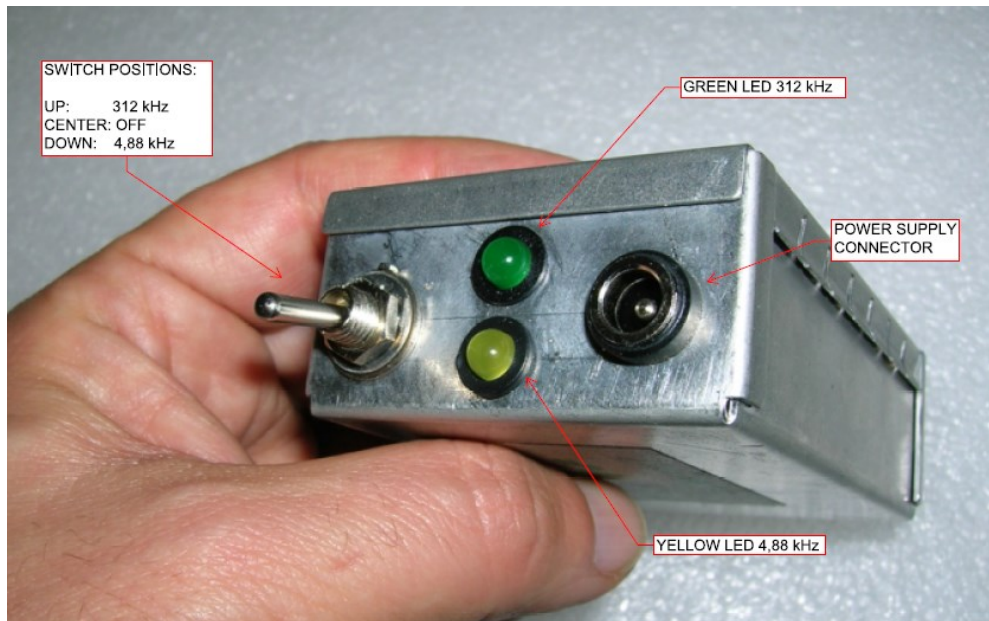
Fig. 3: Detail of the comb generator.
