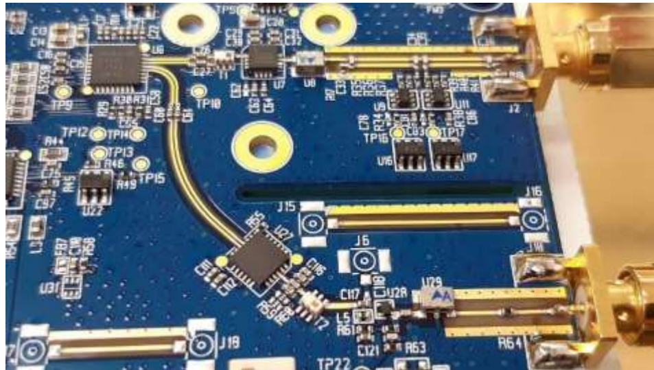
high dynamic range full-duplex DSRC transceivers
